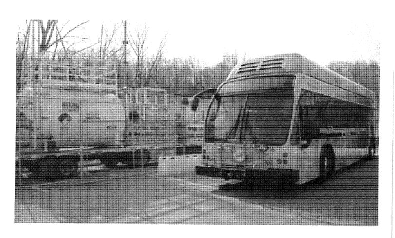
SARTA bus being refueled by a mobile hydrogen refueling at the transit system's offices. (Provided by SARTA)
